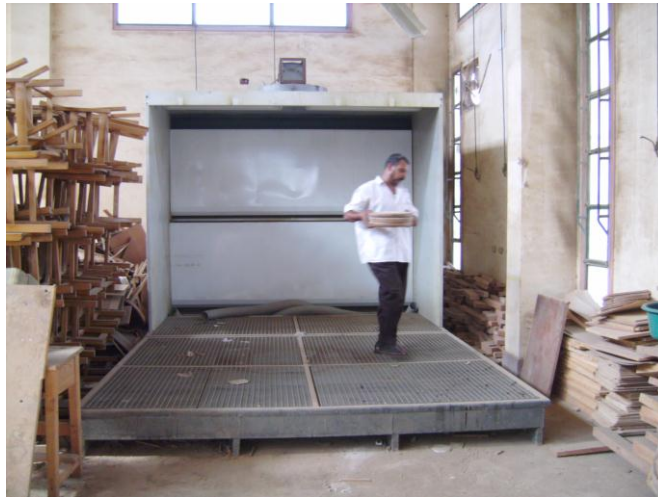
Fig. 17 Cabin for liquid paints Mod. M.I.M SB/3
