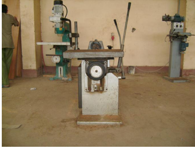
Fig. 13 Mortising Machine T45
